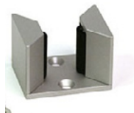
U Guide w/Rollers For 1/2" Material: 3-15-1621-K For 5/8" Material: 3-15-1622-K Use on the inside edge of the opening. Rollers keep panel secure.
