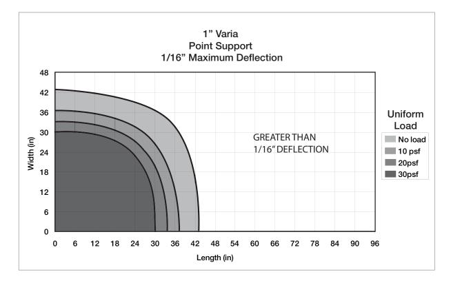
The tables below will provide helpful conversions when using 3form deflection charts. If the desired load is not listed pick the higher value listed. Water load was calculated assuming a fresh water temperature of 77°F (25°C). Snow load was calculated assuming a worst case scenario of 50% density snow.
