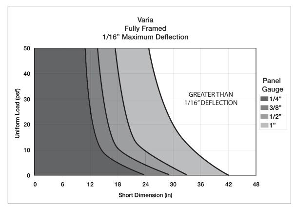
presented in the chart are uniform static loads on the surface of the panel.
