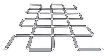
Screw standard frame in place on the wall prior to mounting the grid. This will help you to locate the grid on the wall.
