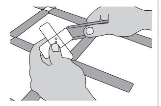
Assemble all the full vertical lengths of the frame and lay them out next to each other. The grid is best assembled on a large table or floor to avoid possible damage during assembly.
