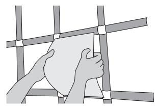
**b** Alternate between horizontal and vertical tiles.
