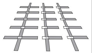
Join the horizontal brackets on one vertical length to the tabs on the next length. For large wall areas it may be easier to assemble the grid in smaller sections, we recommend a full vertical height by 4-6 tiles wide.
