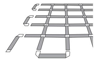
**g** Finished grid should have every second bracket missing around the perimeter.
