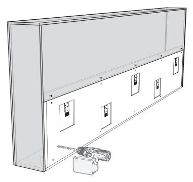
b Drill a ½" access hole in millwork in the matching preferred location to allow low voltage wiring to run to remote driver location.
